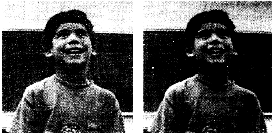
FIGURE 11.19 Left: Reconstructed image using differential encoding at 1 bit per pixel using median predictor and recursively indexed quantizer. Right: Reconstructed image using JPEG at 1 bit per pixel.
