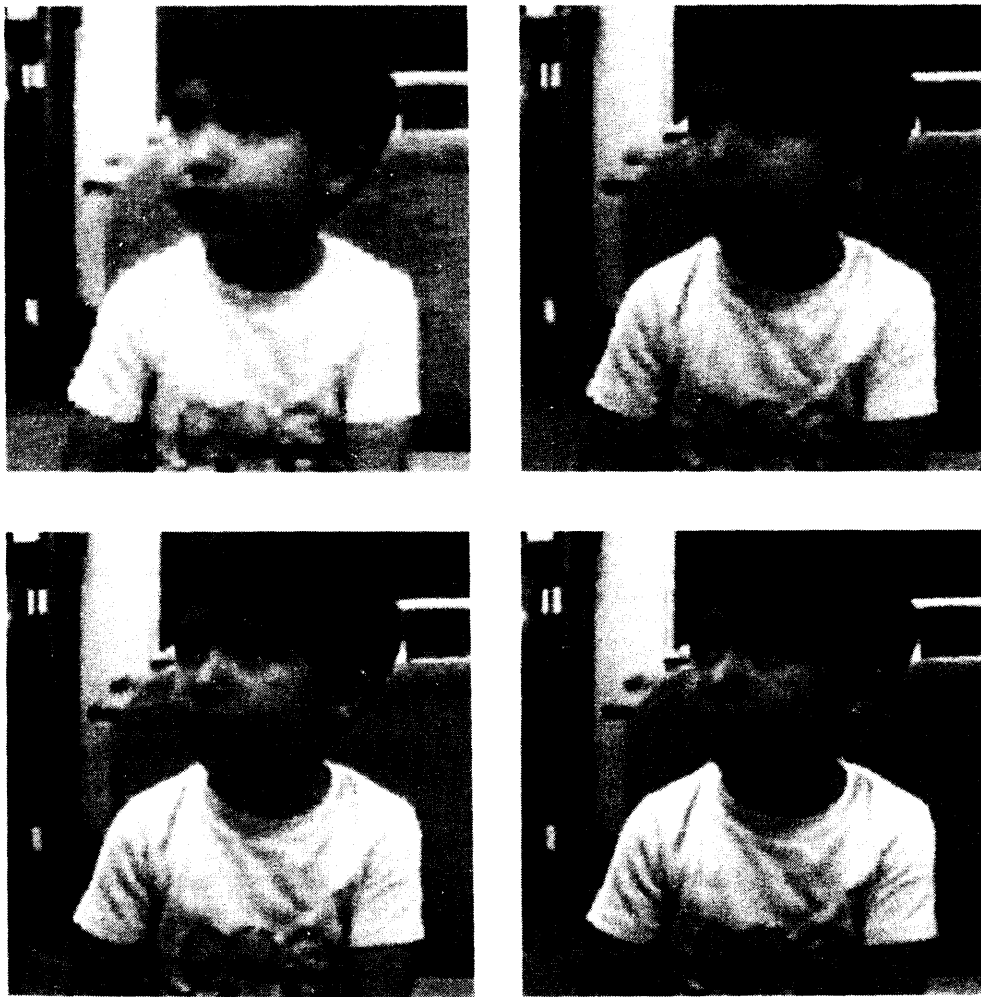
FIGURE 10. 15 Top left: codebook size 16; top right: codebook size 64; bottom left: codebook size 256; bottom right: codebook size 1024.
